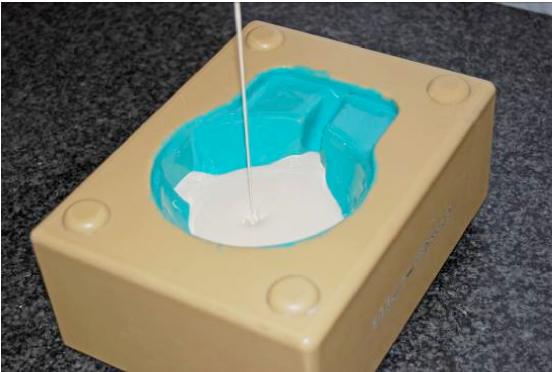
Caption: The latest gelcoat PG-3104/PH-3954, back casting with RAKU-TOOL PC-3415/PH-3915.
