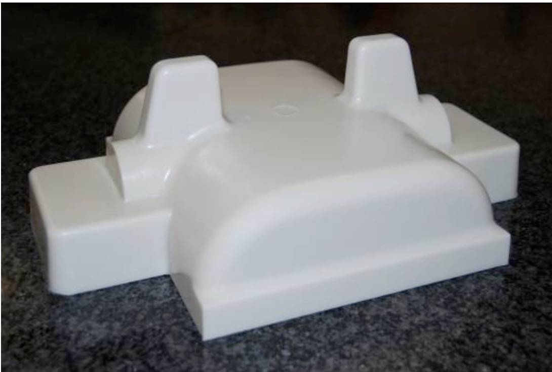
Caption: Model made through face casting with RAKU-TOOL PC-3451/PH-3952, core production with PF-3701-1.
