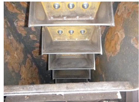
Fig. 2: Conversion of a Chain Bucket Elevator into an AUMUND Coarse Grain Bucket Elevator (BWG-GK, photo AUMUND)
