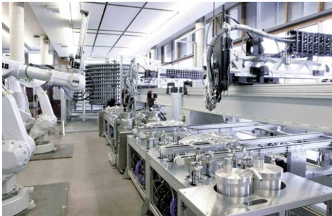
The mixing head MK 600 of the dosing system from Sonderhoff precisely drives the contours of a door module for the sealing with Fast-Cure foam, while the 6-axis robot is in charge of the part handling.
