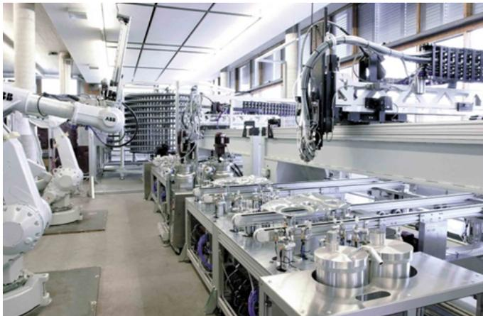
The mixing head MK 600 of the dosing system from Sonderhoff precisely drives the contours of a door module for the sealing with Fast-Cure foam, while the 6-axis robot is in charge of the part handling.
