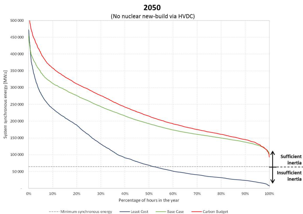
Figure 92: System inertia and minimum system inertia requirement for 2050 (no new nuclear generation integrated via HVDC)
