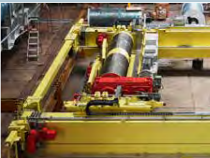
Process crane based on a helical gear unit. The shaft center distances perfectly fulfill the geometric requirements
