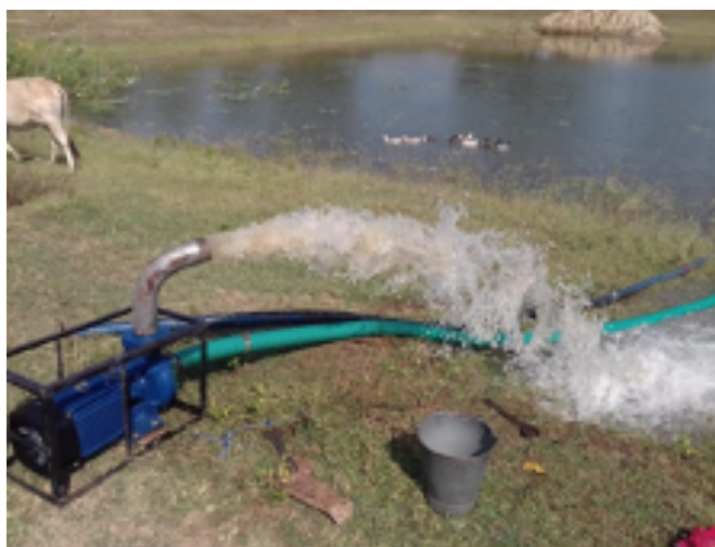
Figure 33 5 horsepower pump powered by the mini-grid used for construction material manufacturing
