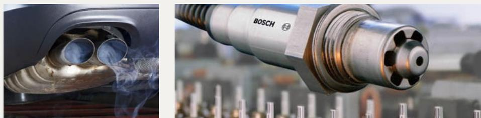
Sensors that detect the presence of oxides of nitrogen (NOx) in exhaust emissions contain both platinum and rhodium and work on a similar principle to the basic oxygen sensor. They are used in conjunction with specialised autocatalysts to control levels of NOx from
