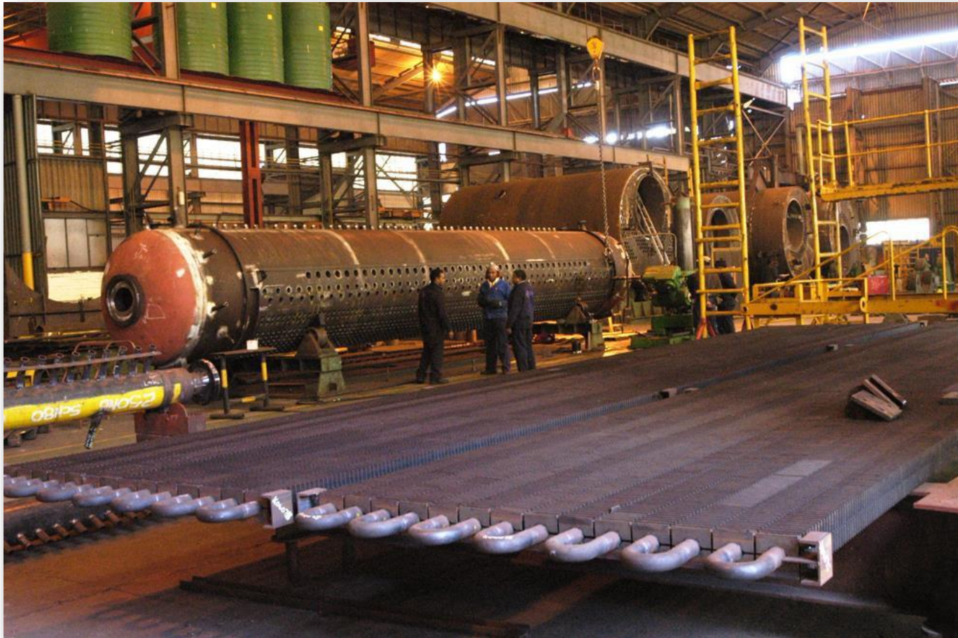
Steam drum and economiser elements
