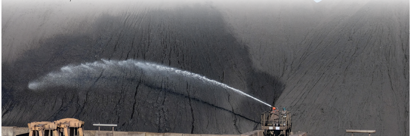
Wetting of iron-ore stockpiles
