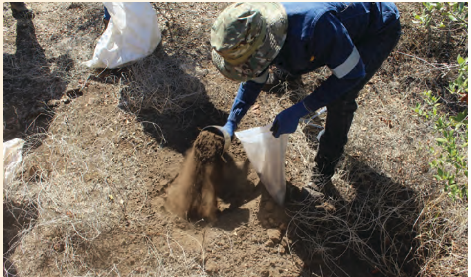
CGS technical assistant collecting a soil sample during a high-resolution soil sampling campaign in the Giyani Greenstone Belt.
