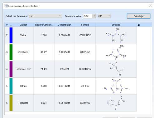
Automatically annotate the peaks and calculate the component areas using the normalized information of the target components
